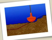
When a bucket over-dredges material, it not only increases necessary bucket cycles, transporting, handling, and processing costs; but it also leaves a hole that often times needs to be filled
