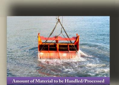
surface the water can then drained from the bucket prior to being dumped into the scow.
